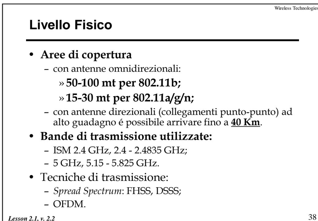
**Livello Fisico****Frequency Hop Spread Spectrum**
